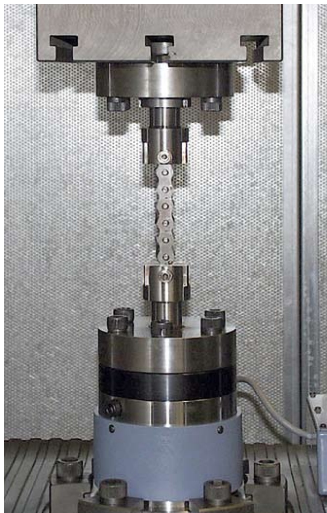
Quality checks with state-of-the-art test stands: fatigue resistance test
