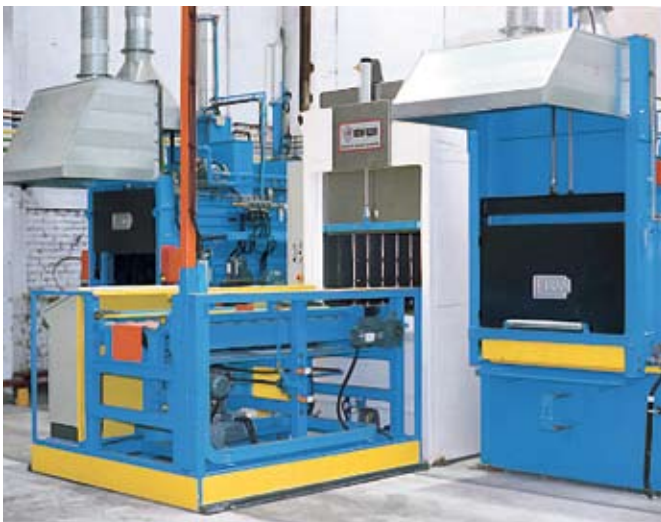
Sophisticated equipment for heat treatment: chamber kiln
